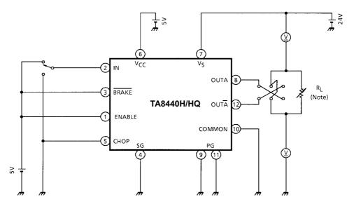
Note: Calibrate I<sub>OUT</sub> to 1.5 / 3.0 A by R<sub>L</sub>.
